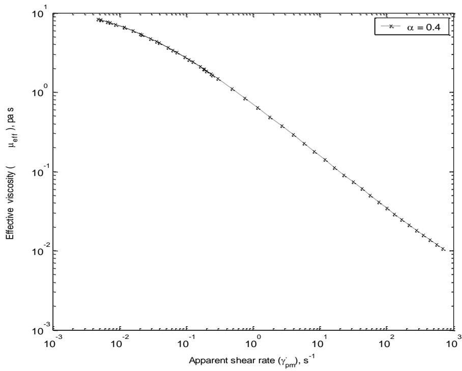
FIGURE 11: Variation of Effective viscosity with apparent shear rate for  $\alpha = 0.4$
