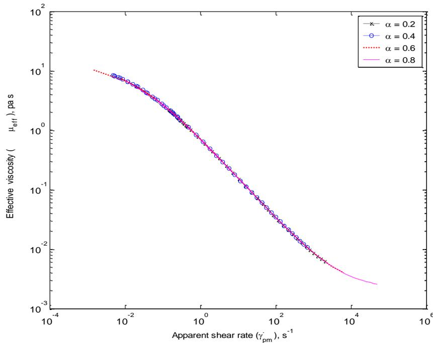
**FIGURE 14:** Variation of Effective viscosity with apparent shear rate for  $\alpha = 0.2$  to  $0.8$
