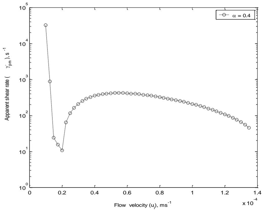
FIGURE 5: Variation of apparent shear rate with flow velocity for  $\alpha = 0.4$
