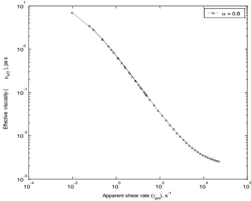
**FIGURE 13:** Variation of Effective viscosity with apparent shear rate for  $\alpha = 0.8$
