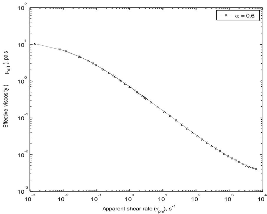
**FIGURE 12:** Variation of Effective viscosity with apparent shear rate for  $\alpha = 0.6$
