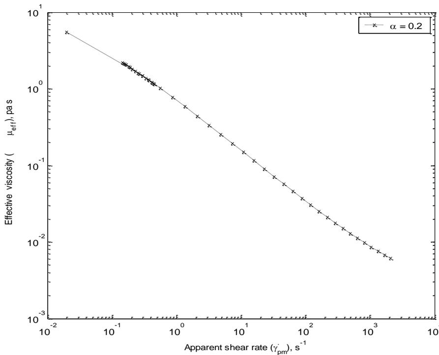
**FIGURE 10:** Variation of Effective viscosity with apparent shear rate for  $\alpha = 0.2$
